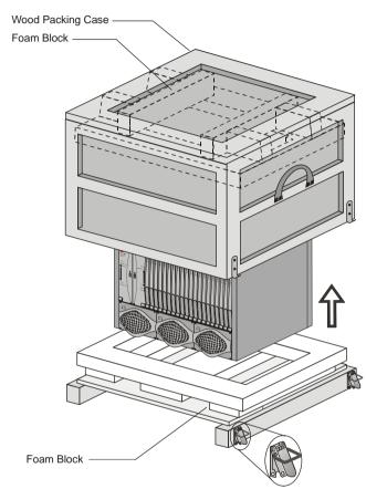
3. Release the clasp locks at the bottom, and lift the MGC+100 top cover.
